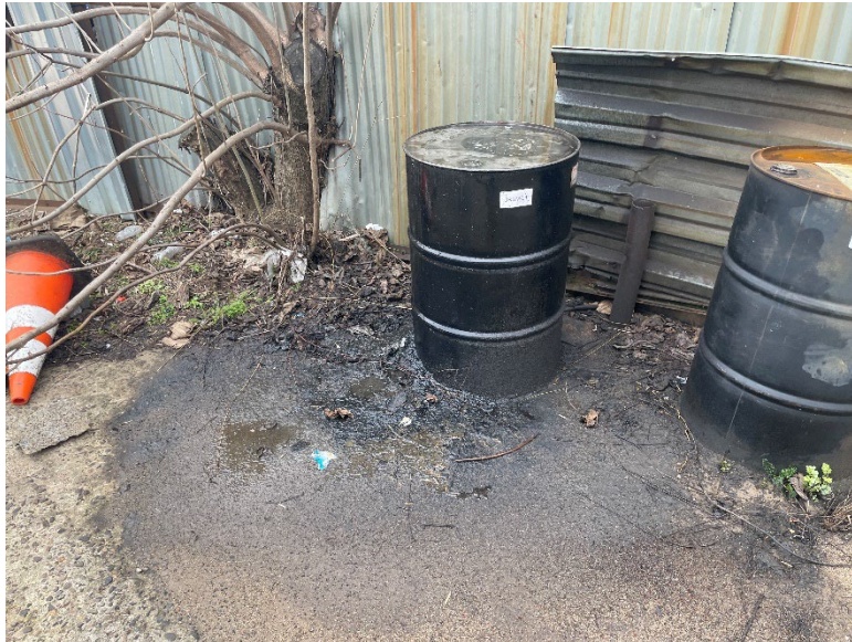
Surficial staining on concrete around DRUM-01 on Block 324
