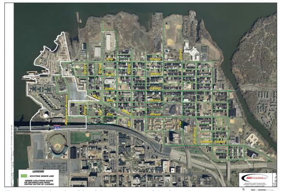
Figure 8 Existing Combined Stormwater and Sanitary Sewer
