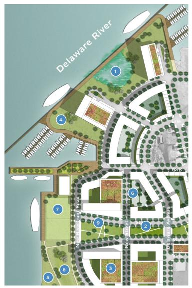
I. Constructed wetlands store and filter excess stormwater, permit infiltration, and enhance biodiversity.
